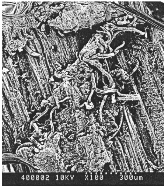
Fig. 2. Scanning electron micrograph of the entanglement of fibres and wood cells immersed in a matrix of molten cell interconnecting material generated by vibration-induced wood welding
