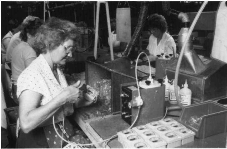
Fig. 3. The bench use of a dispenser for the application of cyanoacrylate to an external light switch to bond the cover to the switch base
