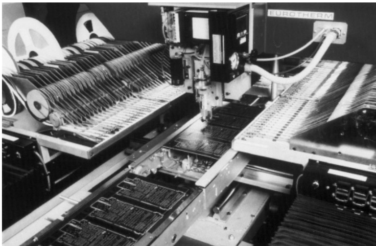
Fig. 2. A typical installation of an automatic machine for placement of components on to printed circuit boards. In the centre can be seen the mounted syringe for automatic application of the adhesive
